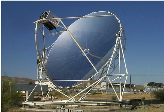
Point focus parabolic mirror with Stirling engine at its center and its solar tracker at Plataforma Solar de Almería (PSA) in Spain
