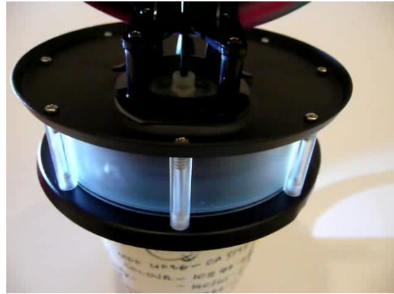
Video showing the compressor and displacer of a very small Stirling Engine in action
